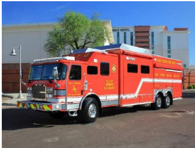
Salt River - Scene Support 294 - 2022 E-One Typhoon - rehab area, cascade and compressor unit, toilet and wash area, awnings, slide down rear stairs for roof top access to storage, light tower
