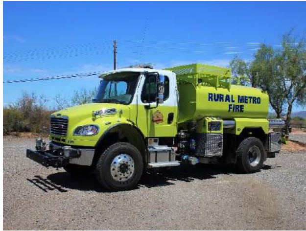
Rural Metro - Tender 826 - 2021 International M2-106 4x4 built by Truck Works. 500gpm pump and 2100-gallon water tank
