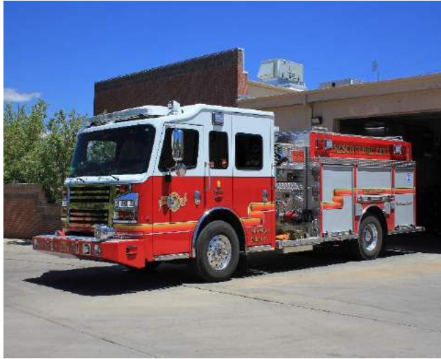
Prescott - E71 - 2021 Rosenbauer Commander 1500gpm 500gwt 20gfta 20gftb
