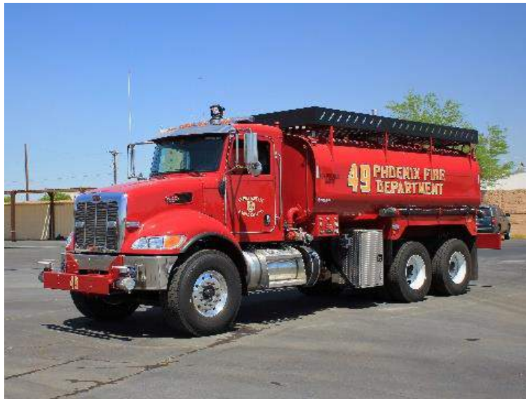
Phoenix Tender 49 - 2021 Peterbilt 348 built by Interstate Truck Bodies. Darley 500gpm pump and 4000-gallon water tank
