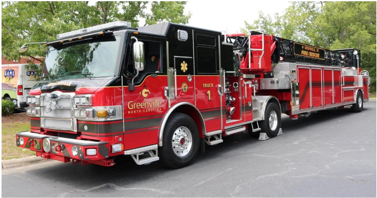
Photo by Robert Reed Jr. Greenville Fire/Rescue (Pitt County, NC) Truck 1 2020 Pierce Velocity Ascendant 107' Heavy-Duty Tiller Aerial Ladder
