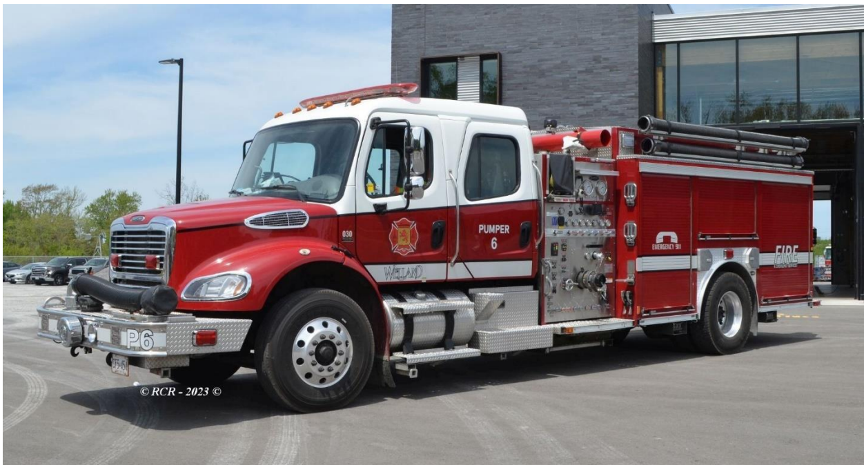
Welland Pumper 6 - 2008 Freightliner M2 112 / E-One 1250/894 SO#134911
