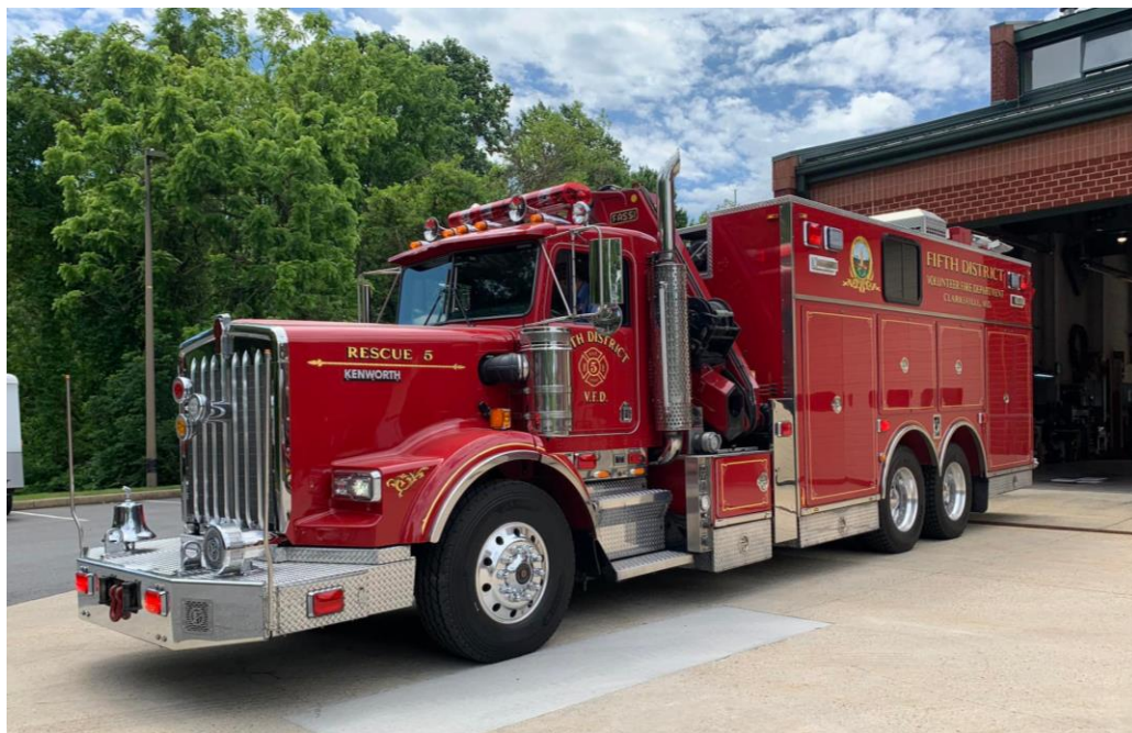
2004 Kenworth/2005 Pierce Walk-In Rescue Crane Ex - Rescue Squad 5 Formerly of Fifth District Volunteer Fire Department, Clarksville MD (Howard County, MD) Now serving Bell Arthur Fire Department, Bell Arthur, NC (Pitt County, NC) as Rescue 5206 850 GPM Portable Pump, 48 ft Hydraulic Fassi Crane, (Has Additional Manual Extensions capable of reaching 67ft) Photo by Robert Reed Jr.
